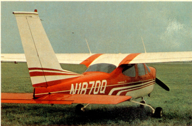
RG is as clean and uncluttered looking from the back as from the front. Fully cantilevered wing, positioned behind the pilot, has almost 30 square feet of flap.
